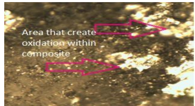
Fig 16: Microstructure of Sample D
