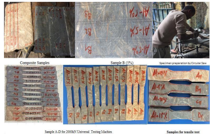
Fig 6: Specimen identification codes (User's code) for tensile test on UTM-2000kN
