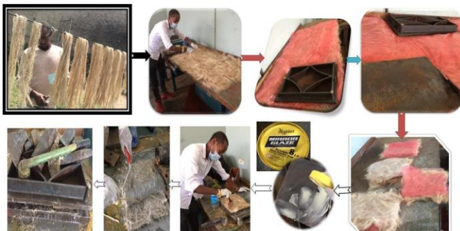
Fig 3: Banana fiber reinforced polymer composite fabrication procedures
