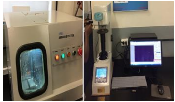
Fig 7: Abrasive cutting in action (RB-203), Micro-hardness measurement under Vickers Hardness Tester (HVS-50)
